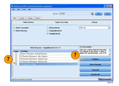
**8.** Use the default values in the Compliance Mode to run the tests for compliance with the standards.
