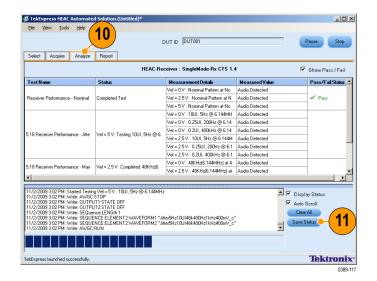
The single mode receiver tests are run at three terminal voltage levels (VeI): 0 V, 2.5 V, and 5 V.
