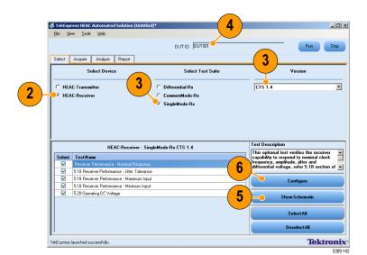
7. Use the default values in the Compliance Mode to run the tests for compliance with the standards.
