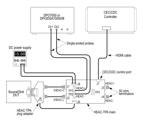
**NOTE.** Use two probes for DC voltage measurement. Use the differential mode configuration for other measurements.
