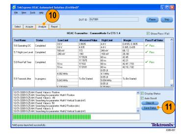
**12.** Follow the on-screen prompts. For the Rise-Fall Time test, configure the DUT to transmit an MLT-3 signal and click **OK**.
