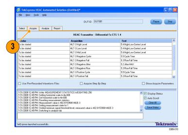
4. Click the Analyze tab when the tests are running to view the status and progress of the tests. The application checks to see if the device has passed the test. The Status Messages window time stamps all runtime messages and displays them.
