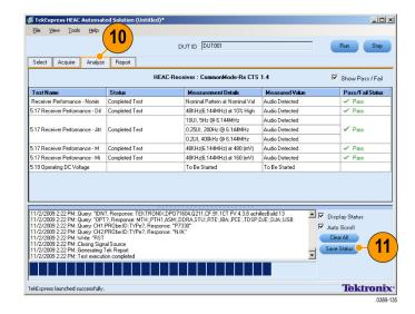
12. As the selected tests are executed, the application prompts you to verify the audio response from the DUT. Click **Detected** or **Not Detected** as appropriate for each test.
