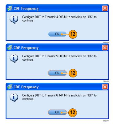
13. The IEC Stream Verification test is run under three conditions: with +5 V power turned on and ARC activated, with +5 V power turned off, and with +5 V power turned on and ARC not activated. Follow the prompts and click OK.
